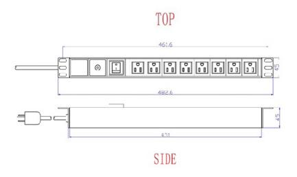
Print on the power cord jacket: (UL) E308842 SJT 3/C 14AWG(2.08sq.mm) 105C 300V VW-1 105540-001
